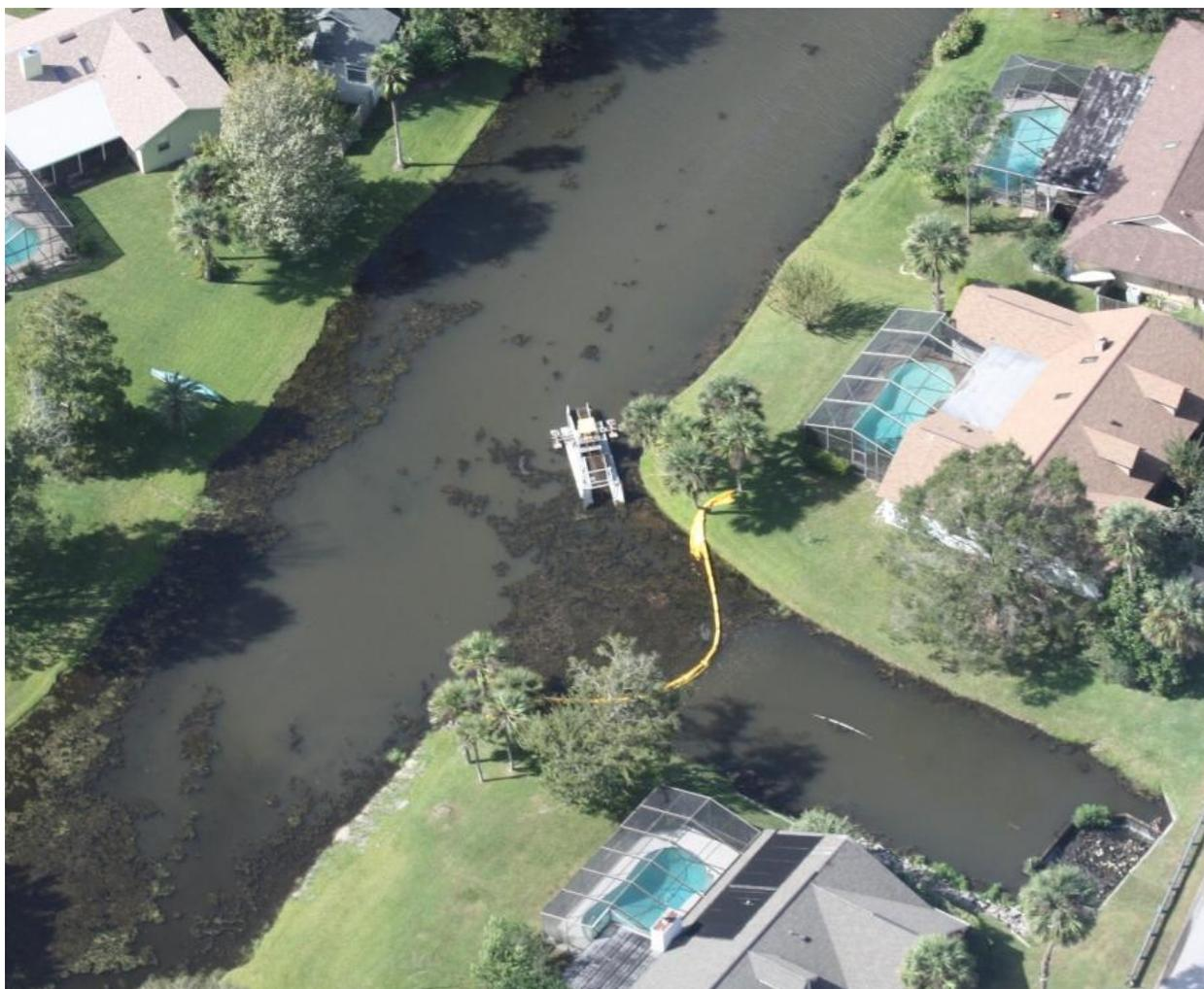
Figure 1-12. Harvester Used for Lyngbya Removal.
